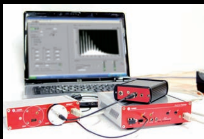
Set-up for SiPM testing & characterization
